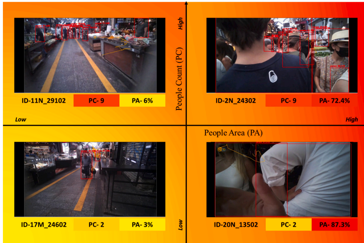
Fig. 10. Classification of overcrowding (bottom left: low People Count and People Area; top left: high People Count and low People Area; bottom right: low People Count and high People Area; top right: high People Count and People Area).
